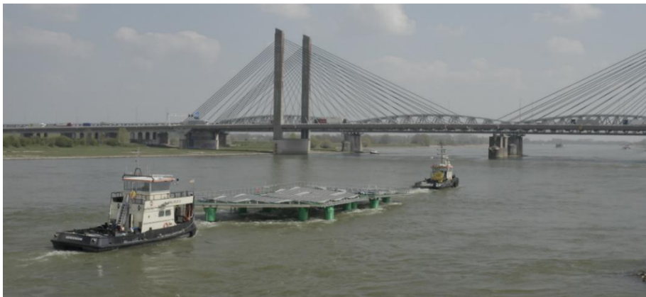
Figure 1: The SolarDuck platforms under tow
